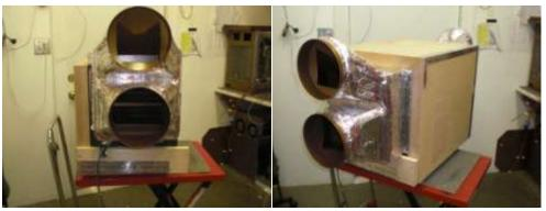
4. Place the top/side panel over the unit with the access opening on the side of the unit where the access panel is.
