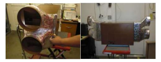
3. Place the unit on to the section that has the bottom and side panels connected, for units that have the probe/remote controller cable coming out of the bottom there is a cut out. Once the insulation box is assembled the area around the opening for the cables needs to be sealed with silicone.
