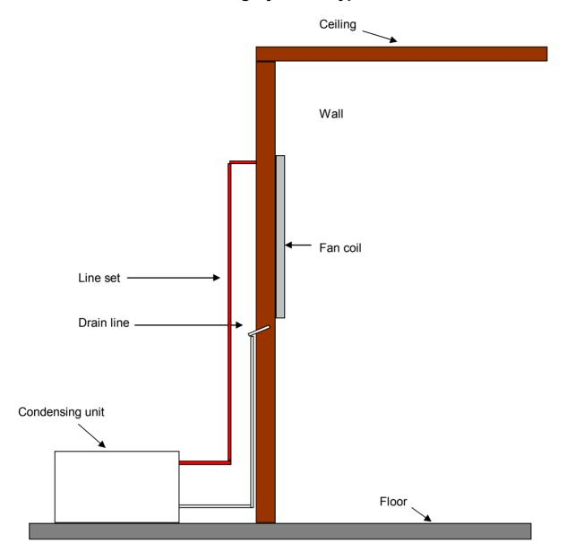
Fan coil is bolted to ceiling. Allow 3" between it and wall for proper air flow. Keep line set as short and direct as possible. Excessive number of turns will cause refrigerant flow problems. This would cause early failure of compressor Drain line must always flow down hill. Return to condensing unit on systems up to 3600 btu or drain to a point allowed by local code.
