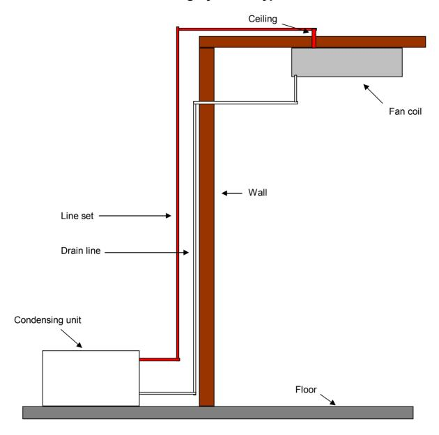
Fan coil is bolted to ceiling in center of room for proper air flow. Keep line set as short and direct as possible. Excessive number of turns will cause refrigerant flow problems. This would cause early failure of compressor Drain line must always flow down hill. Return to condensing unit on systems up to 3600 btu or drain to a point allowed by local code.
