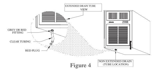
**EXCESS CONDENSATE DRAIN TUBE:** Your unit is equipped with a **Pull-down Drain tube** to prevent condensate overflow. This tube should only be used to temporarily drain excess amounts of condensate caused by excessive moisture laden air entering the enclosure. The source of this air must be eliminated.
